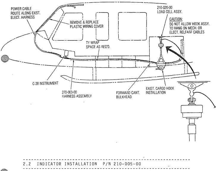
The indicator should be mounted in a position that is convenient, accessible and visible to the pilot. It can be mounted in a standard 2-1/4" instrument hole.
