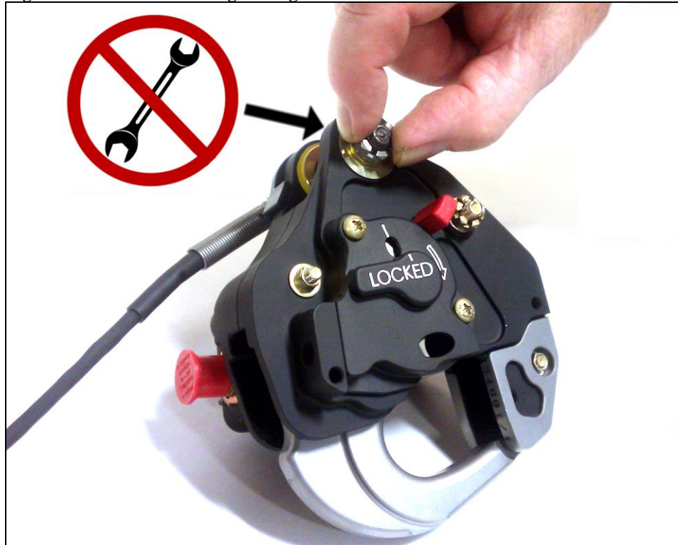
Figure 2.7 Pin Load Cell Tightening
