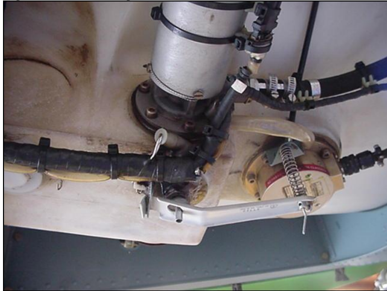
Figure 2.3.1 Removing Control Cable
