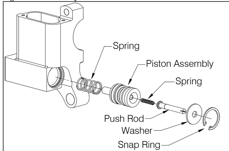
**Figure 12.4 Master Cylinder Piston Seal Orientation**
