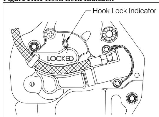
3. Swing the cargo hook and the suspension system throughout their full ranges of motion to ensure the hydraulic hose and electrical release harnesses have enough slack. The hose or harness must not be the stops that prevent the cargo hook or suspension from swinging freely in all directions.
