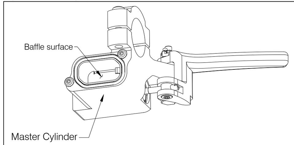
If leakage is noted around any plumbing fittings, the fittings may be tightened until the leakage quits. If leakage is noted around the pistons in either the master or slave cylinders the leaking cylinder must be repaired. See the instructions for repair in this Section.
