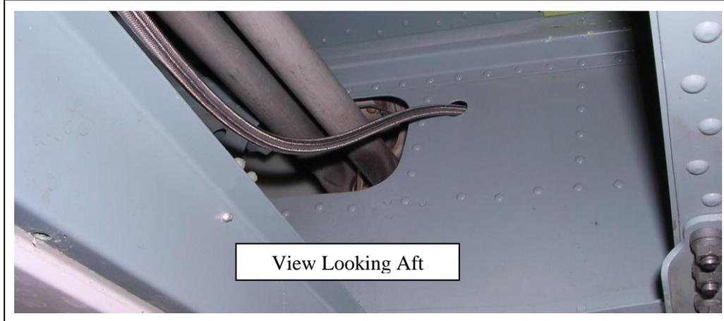
8. Aft of the rear cabin bulkhead pick up the existing electrical harness runs and secure hydraulic hose using ty-wraps. The hose will route outboard of Y400 and follow the cargo hook electrical release harness to the connector bracket.
