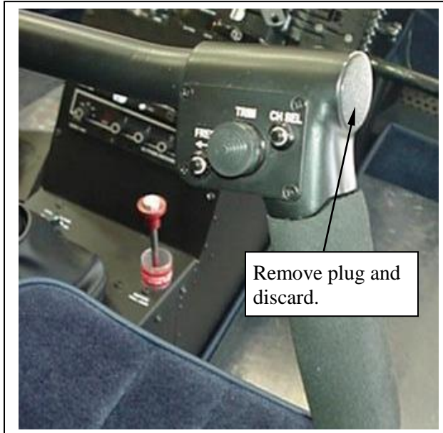
Figure 2-8 Grip Assembly C058, Plug Removal
