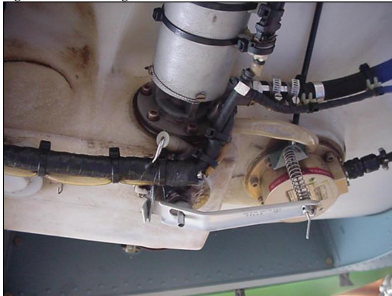
Figure 2.5.1 Removing Control Cable
