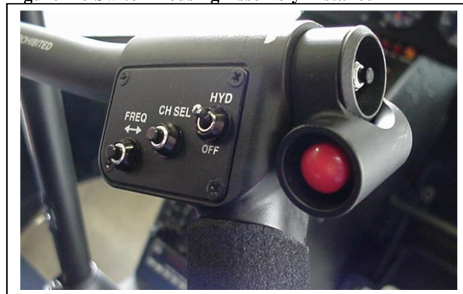
Figure 2-8 Switch Housing Assembly Installed
