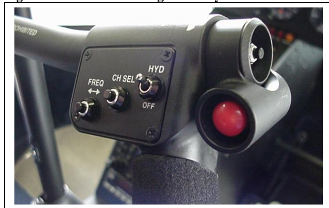
Figure 2.5.7 Switch Housing Assembly Installed
