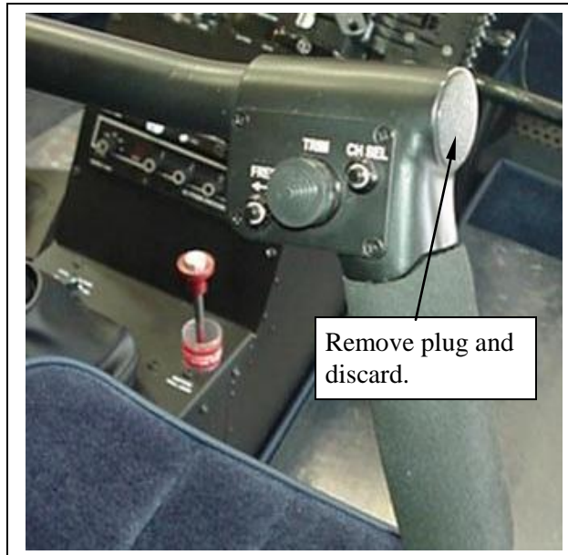
Figure 2.5.1 Grip Assembly C058, Plug Removal
