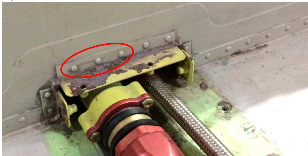
Figure 3.1.2 Brackets and Rivets to Remove (Forward Bulkhead)
