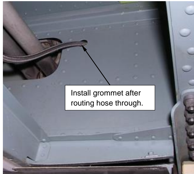
Figure 4.4.7 Hose Routing Through Aft Bulkhead
