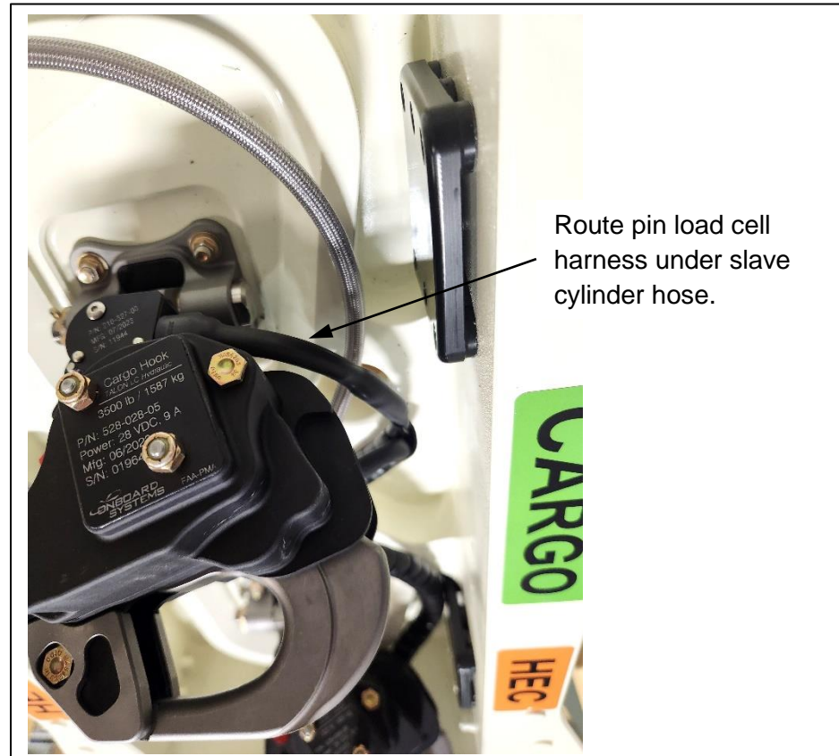
Figure 6.1.2 Pin Load Cell Harness Routing
