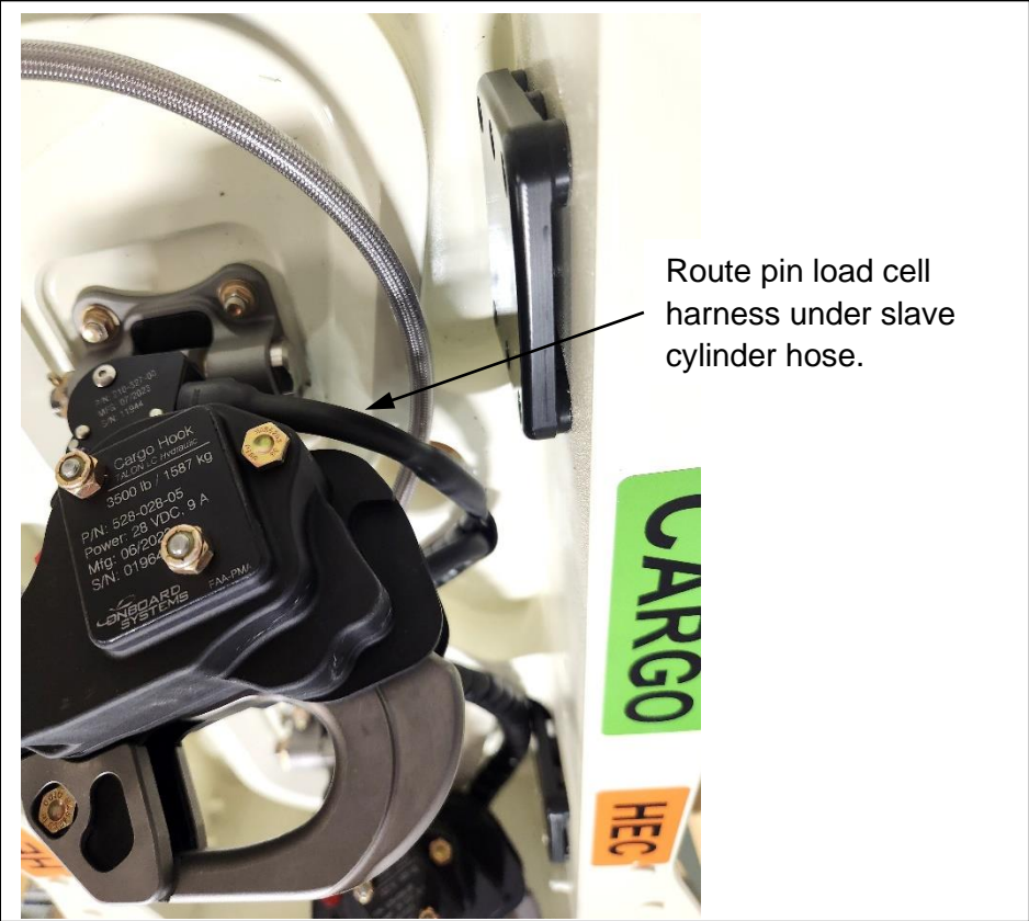
Figure 6.2 Pin Load Cell Harness Routing
