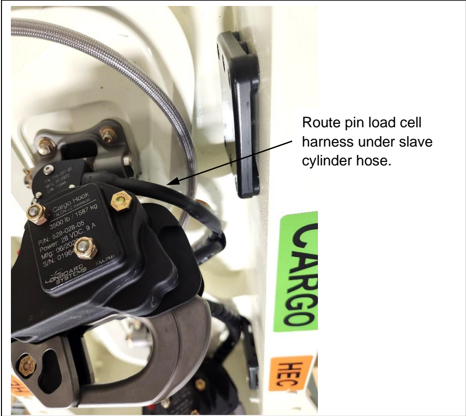
Figure 6.2 Pin Load Cell Harness Routing
