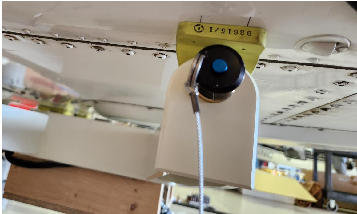
Figure 3.5 Positioning Lug Assemblies with Recommended Frame Support
