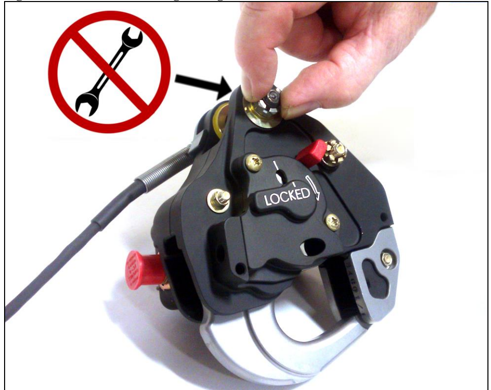
Figure 2.6.3 Pin Load Cell Tightening
