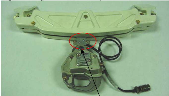
Figure 1. Suspect Part: 210-179-00, E-85 Load Cell
