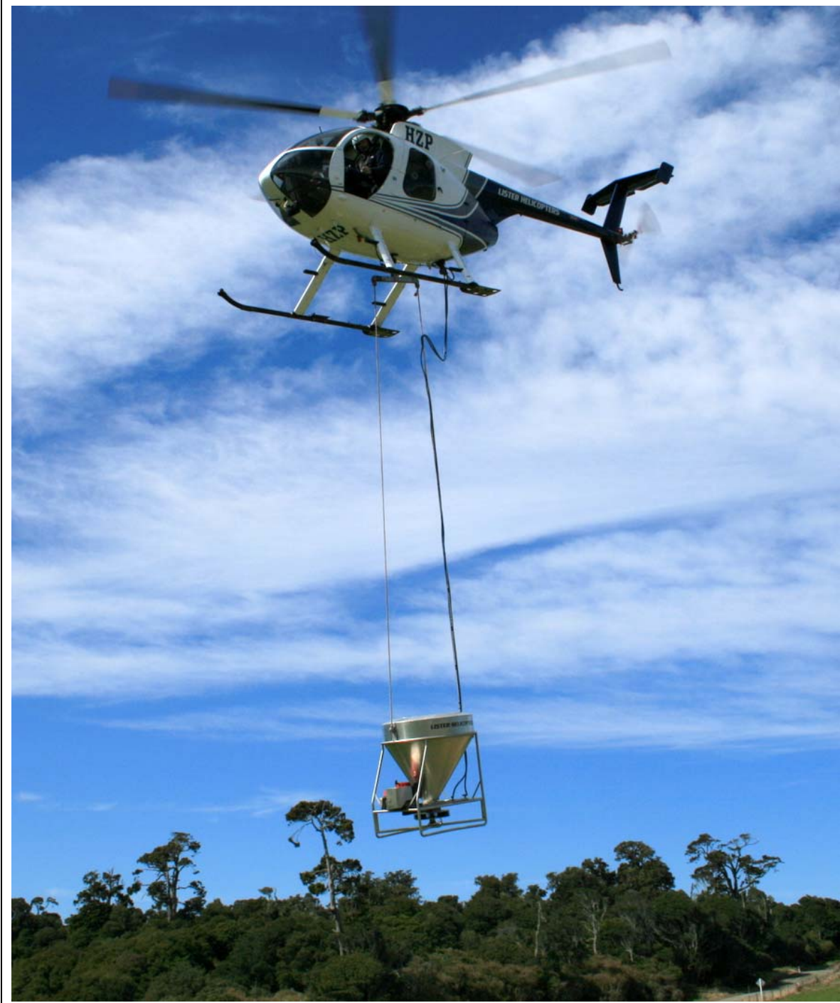
Figure 2 – Fertilizer application using bucket and spreader bar. Photo: Lister Helicopters
