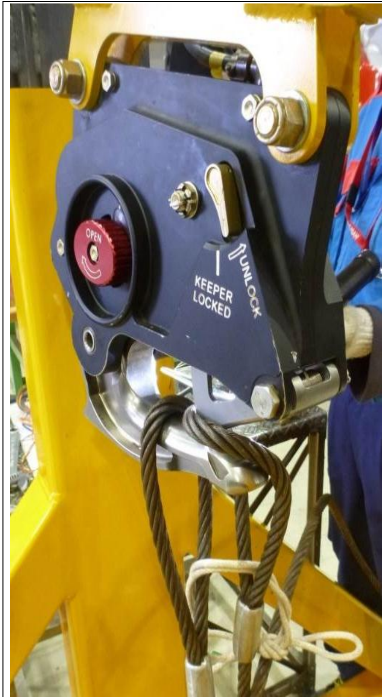
Figure 1 – Failure scenario: Improperly loaded wire sling.
