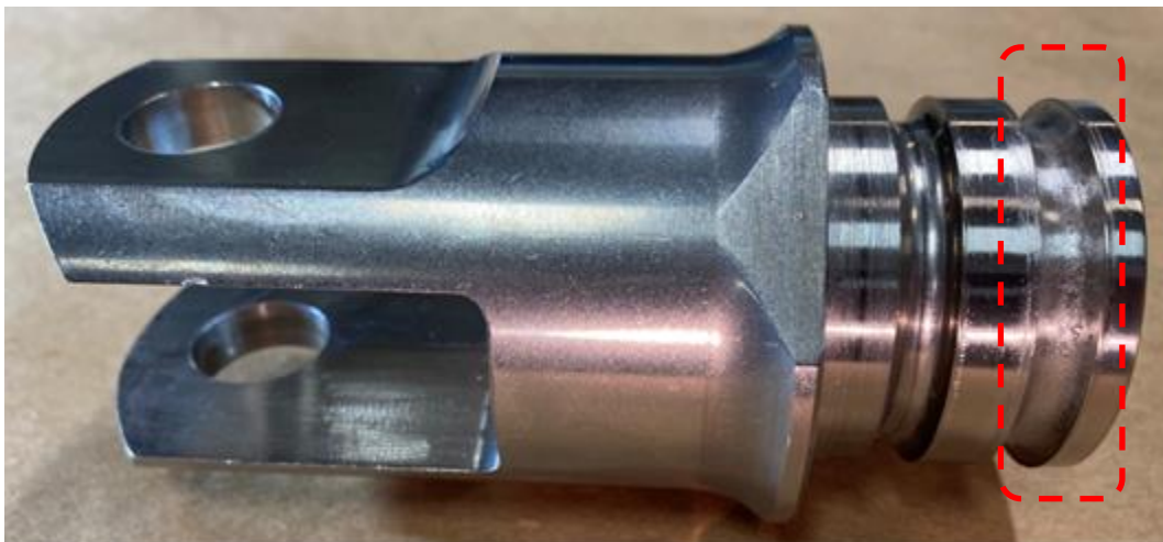
Figure 1 – Worn Bearing Race
